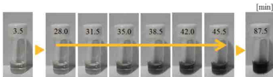
Fig. 6. Time-dependent color of residue in a vial container (Numbers show time from mixing).
