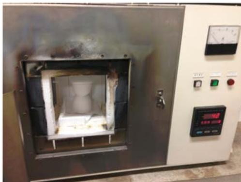
Fig. 3. High temperature furnace. The synthesized powders of electrolyte were calcined at 1400°C for 10 hours.
